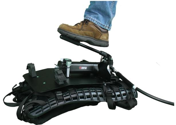
Highly portable and effective hydraulic breaching toolkit in a custom made backpack. Quick disconnect fittings allow operator to switch tools depending on mission. Door pusher, jamb spreader, bolt cutter, and hydraulic wedge can all be powered easily and quietly from dual stage 10,000 psi pump. US made pack has padded shoulder and waist straps for ultimate mobility.
